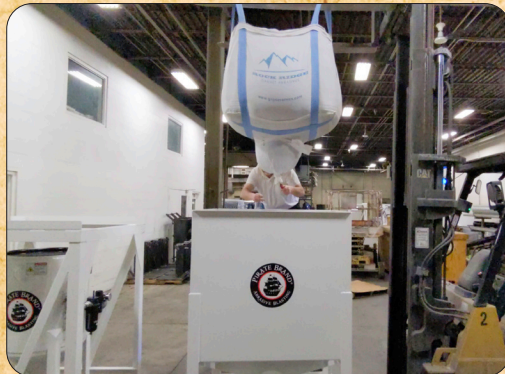
3) Bulk bag is positioned above hopper and prepped for abrasive release.
