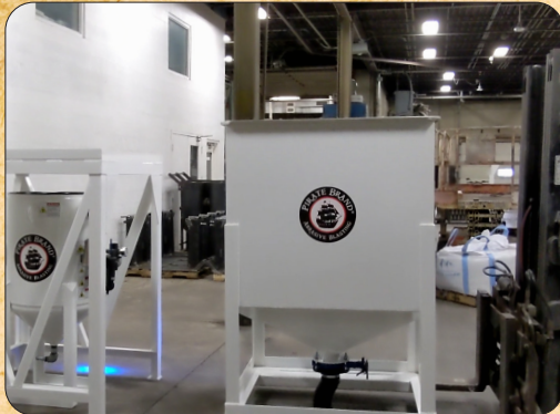
1) Hopper is placed on the ground via forklift.
